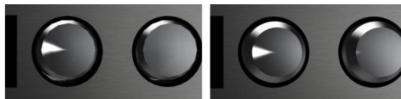
Figure 3: State of the art raytracing technology based on tessellated geometry (left), versus NURBS-raytracing technology (right).
