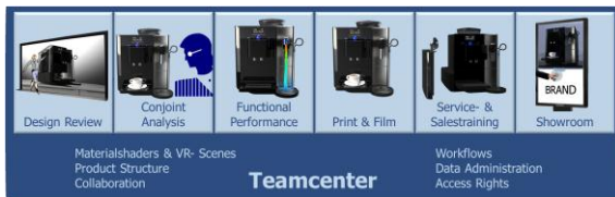
Figure 1: A VR-Process fully integrated into the PLM backbone utilizes the base technology of the PLM system for workflow support, updating and revision management, access rights control, collaboration and conferencing etc.
